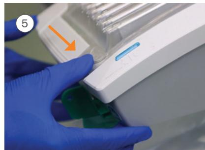
Push the **cassette down** and the **latch forward**, ensure location by checking that the **latch is flush** with the front of the InterCooler™ housing (see fig.1 below)
