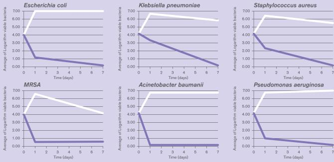
The addition of Silver Ion anti-microbial additive to Intersurgical breathing system tubing greatly reduces the viable microbial count level over time. The tubing has demonstrated a long lasting anti-microbial affect against a broad range of micro-organisms responsible for Hospital Acquired Infections. References: 1. Intersurgical Ltd. Certified Independent Test Results, 2019.
